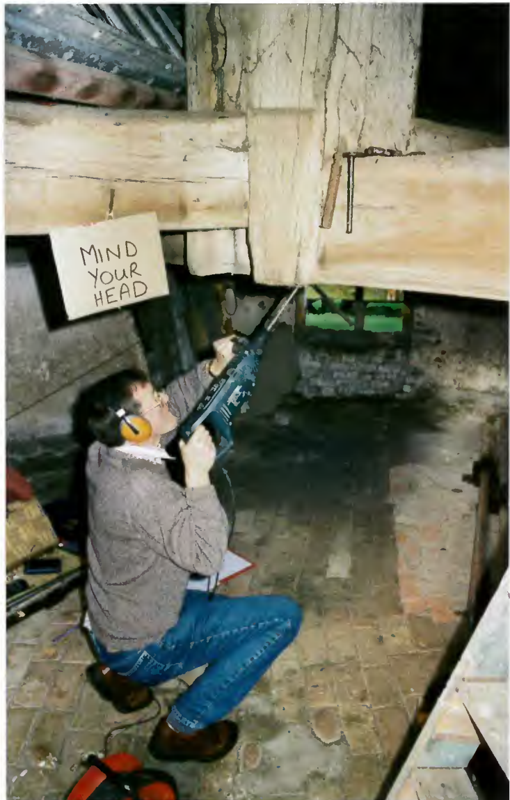
Martin Bridge taking a core from the base of the post at Drinkstone
