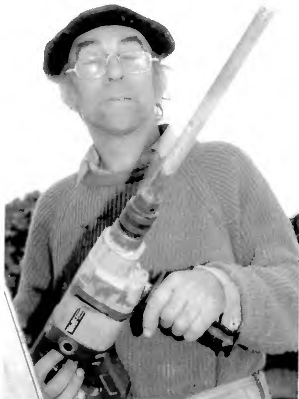
Chris Hullcoop with the hollow drill made from a chairleg
