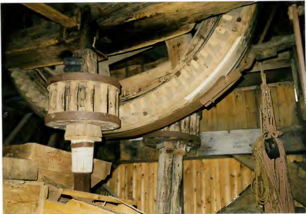
St Annaland post mill: the direct drive off the brakewheel to the two pairs of stones
